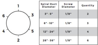
4. Always start the first fastener at the largest radial gap between fitting and duct. Be sure to achieve even distribution around the circumference.
