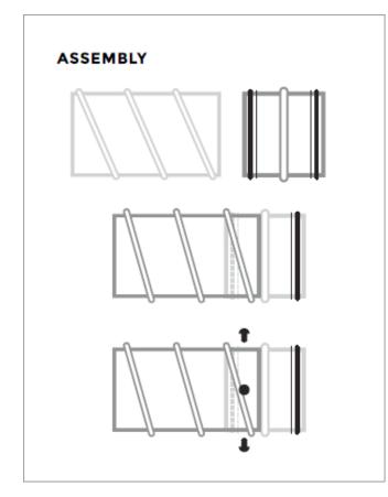
1. Place the hemmed end of the fittings in the spiral pipe, then apply pressure and the fitting will slip into place, stopping at the bead/pipe stop.
