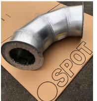
**Exceptional Thermal Performance!** Our standard product uses the KoolDuct® 45mm board. This product has an R-value of 12.0. It is machined to fill a 2" annular space in our double-wall construction, and our process eliminates all potential thermal gaps. This is 50% more thermal performance in a 2" insulation product than you would get with fiberglass or elastomeric insulations.
